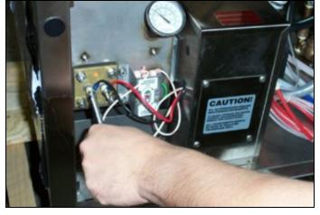
Removing the heater nuts.
